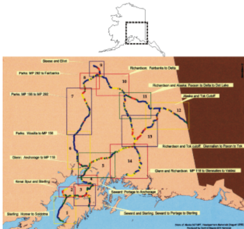
Figure 2. Map of the main surfaced roads in Alaska. The sections in red are at risk due to permafrost; the sections in blue are not. 5
